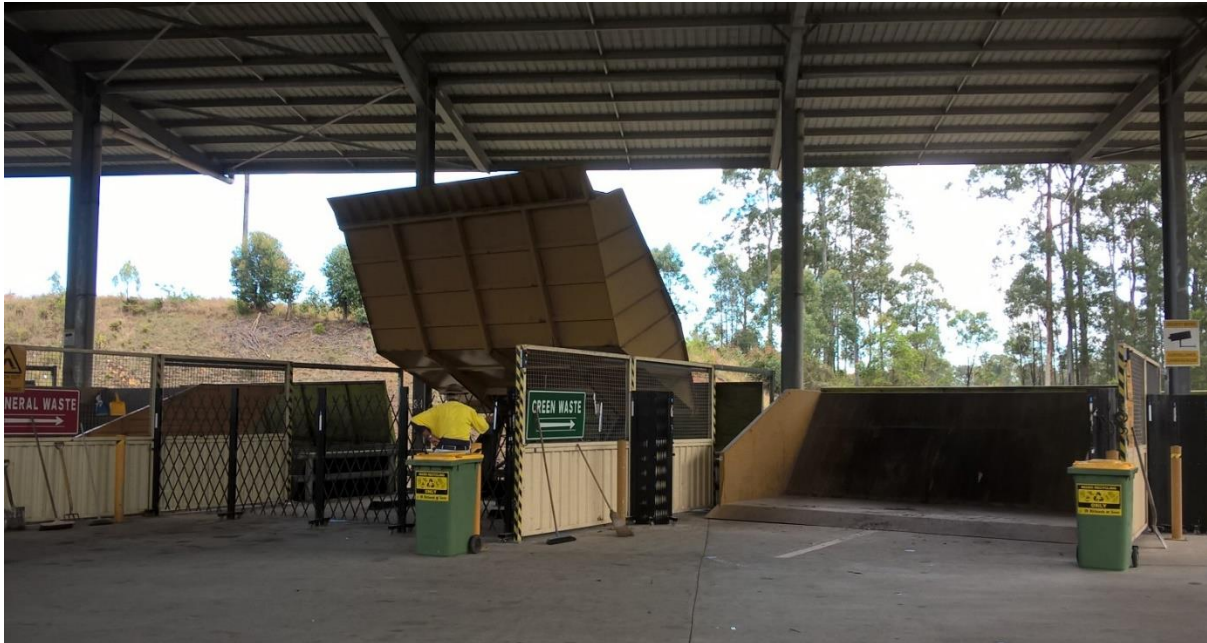
Figure 5-3 Hydraulically operated tipping bins in operation at MidCoast Council's waste facility
